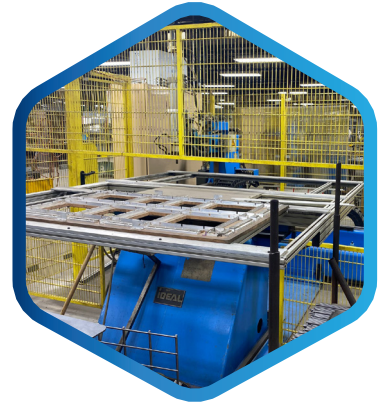
CNC Position Welder
